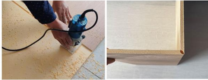
Back grooves can be 90° Angle wrap column wall
