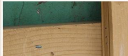
02 Secure the wooden keel with steel nails
